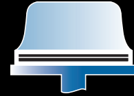
Cross section of Trelleborg® Press-on Solid Tire
